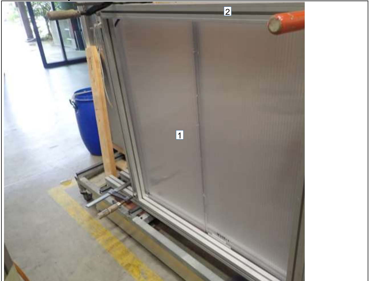
Figure 1 The test specimen (1) in a frame made of aluminium profiles (2).
